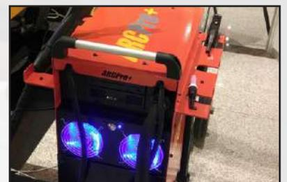
Arcpro+ offers versatile cost-effective and safe high quality welding training. Arcpro+ enables wide variety of welding working conditions to improve hand skills thanks to high fidelity motion tracking system.
